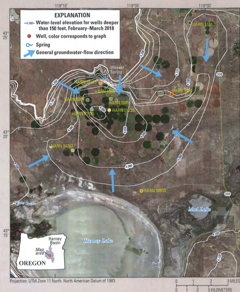
Locations of selected groundwater-level sites and groundwater-level contours (in feet above North American Vertical Datum of 1988) in the Weaver Spring/Dog Mountain area, Harney Basin, southeastern Oregon. Contours from Gingerich and others, 2021. Background aerial image source: GoogleEarth™ 2019.
