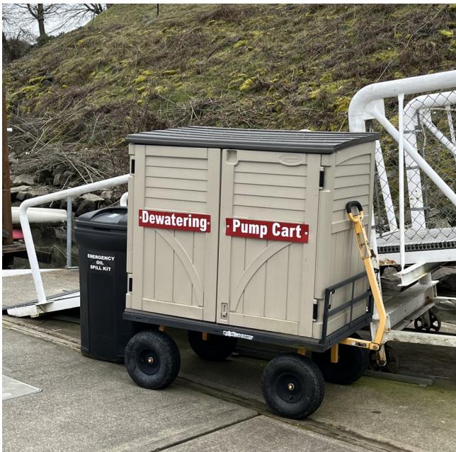
Emergency boat de-watering pump cart
