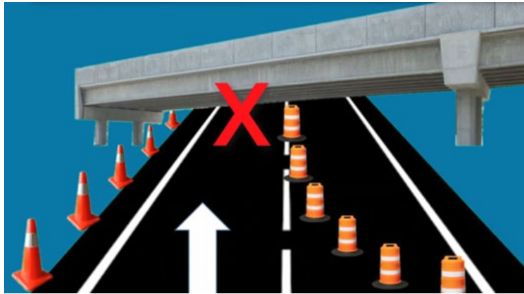
Figure 9: A lane closure/lane shift under a structure can result in lower vertical clearance
