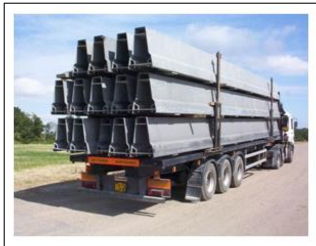
Figure A-1: Steel Barrier in Transportation
