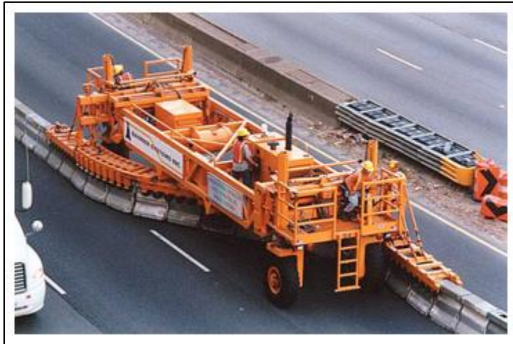
Figure A-1: Concrete “Zipper” Barrier
