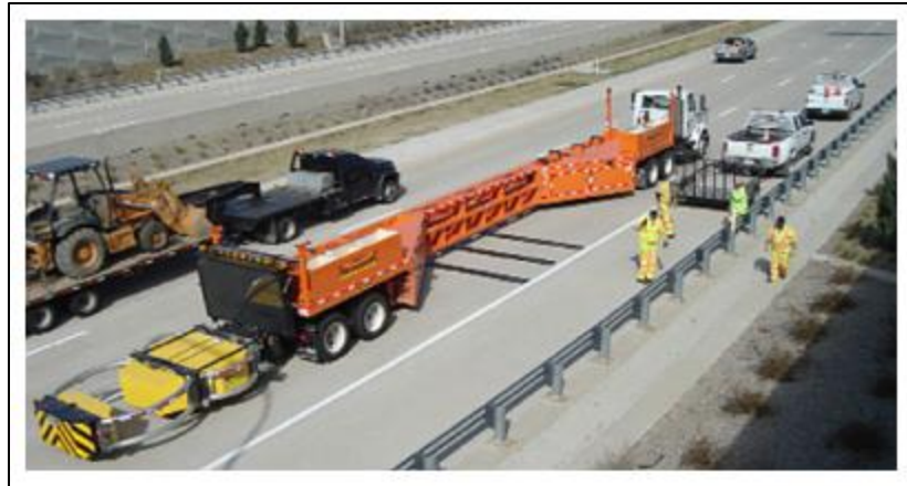
Figure A-2: Mobile Concrete Barrier
