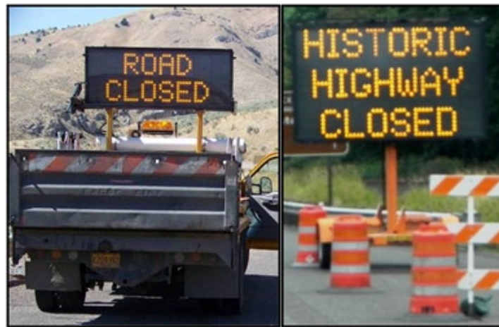
Figure 1 - Example of a truck mounted PCMS (left) and a trailer mounted PCMS (right).
