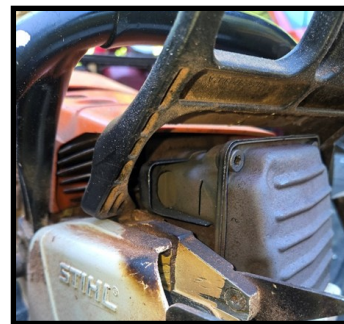
Stihl MS461 with Modified Exhaust
