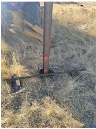
Media 69: PLT-02 Uplift Test Example
