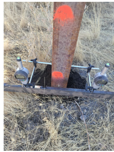
Media 70: PLT-02 Uplift Test Example
