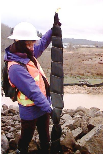
Chitosan Sock (Left) and Treated high turbidity sample after five minutes (Right)
